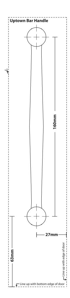
Cut out selected handle template and place on door as per recommended drawing (dotted lines are indicative only measurement prior to drilling is advised)
