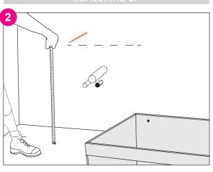
Remove doors & drawers and drill holes for plumbing in the back panel and/or base of the cabinet with an appropriate sized hole saw. Pre-drill screw locations for fastening to wall in step 4
