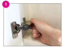
To separate the softclose mechanism from the hinge use two fingers and gently pull from the back to the front.
