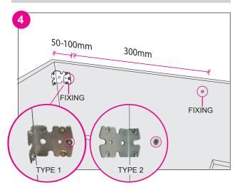
Securely fasten cabinet to wall through the back, no further than 100mm from each side of the cabinet. Upper fixings should be no lower than 50mm from the top of the back. Where possible, fasten cabinet through steel bracket in the top corner of the unit. Note: For cabinets over 900 wide you must provide additional fixing points evenly spaced at 300mm.
