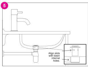
When fitting waste to basin do not overtighten or the basin may be damaged. Use suitable overflow waste and align the slots with the internal holes in the basin. Ensure that no excess silicone or putty is obstructing the water flow.
