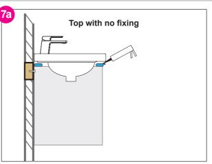
Position the top so that it has an equal amount of overhang on each side and use a level to ensure the vanity top surface is level. Note: If the vanity is being installed in a corner, a packing strip is required and basin location will vary.
