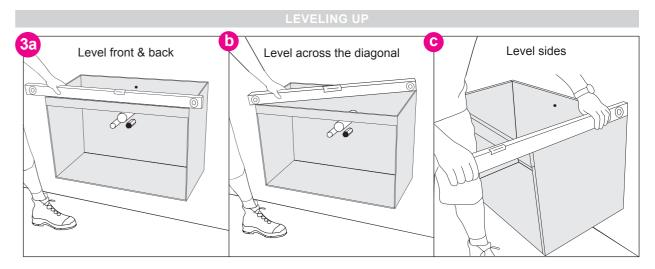
Note: Floor standing vanities should likewise, be checked for sitting level plumb and square and suitably packed to achieve this. Fix to the wall to secure either through the back rail or back panel.
