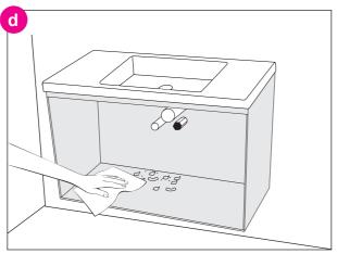
Clean away all building residue from the cabinet. Take care to dry any spillage or leakage of water on or inside the cabinet during installation. Note: Ensure drawer runners are free of building
