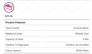
The basin must be sealed to the top with an acetic cured silicone sealant.
