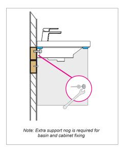
Position the top so that it has an equal amount of overhang on each side and use a level to ensure the vanity top surface is level. Note: If the vanity is being installed in a corner, a packing strip is required and basin location will vary.
