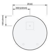
**IMPORTANT NOTE:** Throughout this guide, tolerance for mirror size may vary by ±1mm, tolerance for bracket position may vary by ±5mm. Please read the installation manual for detailed information on installing the product. St. Michel pursues a policy of continuing improvement in design and manufacturing of its products. The right is therefore reserved to vary specifications without notice.
