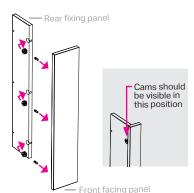
Screw cam dowls into trimmed outward facing panel. Knock cams into rear fixing panel + assemble.
