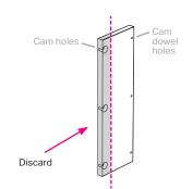
Trim your front facing spacer to fill gap. Cut away cam holes, leave cam dowel holes to connect to rear fixing panel. Note: Adjust trim angle to match any walls out of plumb.
