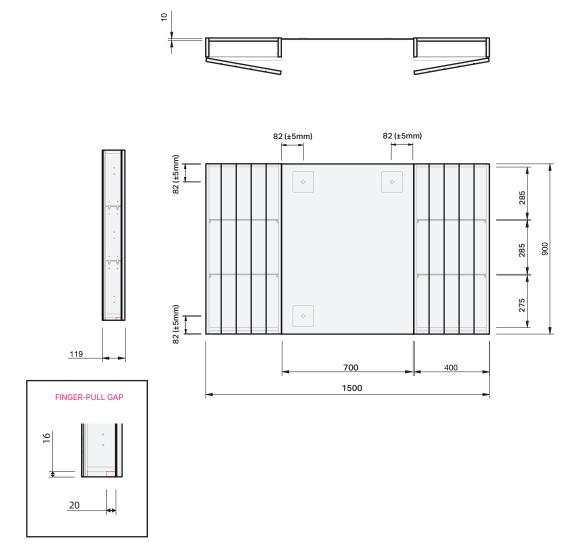
**IMPORTANT NOTE:** Throughout this guide, dimensions may vary by ± 2mm. Tolerence for bracket position is ± 5mm. Please read the installation manual for detailed information on installing the product. St. Michel pursues a policy of continuing improvement in design and manufacturing of its products. The right is therefore reserved to vary specifications without notice.
