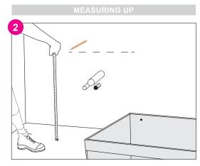
Mark the position of the top of the vanity - factor in the top/ basin thickness to get the correct height. Use a single screw in center of vanity to hold it in place.
