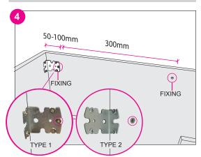
Securely fasten cabinet to wall through the back, no further than 100mm from each side of the cabinet. Upper fixings should be no lower than 50mm from the top of the back. Where possible, fasten cabinet through steel bracket in the top corner of the unit. Note: For cabinets over 900 wide you must provide additional fixing points evenly spaced at 300mm.
