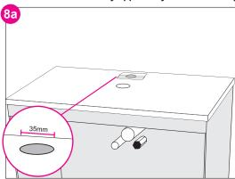
Decide on the location of your taphole and measure out position. Tapholes should be drilled with a sharp Bi-metal hole saw. The drilling is done in three steps. Cover the area you plan to drill with masking tape. Drill a pilot hole through the counter top at your center point. This hole should be just slightly smaller than the size of the pilot bit of your hole saw.
