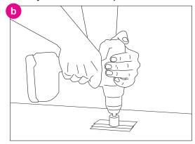
Using this hole as a guide, use a sharp hole saw to cut the hole to 35mm for a standard taphole size. Note: Use a very sharp hole saw to prevent damage to your top.
