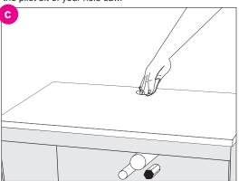
Remove tape & sand the edges of the holes with 240 grit to remove any sharp edges.
