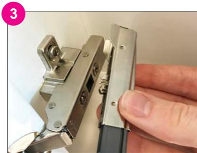
To re-install insert tongue and hooks into cut out, gently pull forward and press rear back into position.
