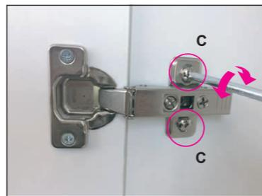
Loosen the top and bottom screw **C** on each mount plate, adjust door height by moving door up or down, then retighten **C** screws
