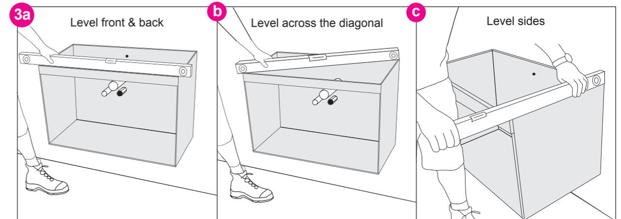
Note: Floor standing vanities should likewise, be checked for sitting level plumb and square and suitably packed to achieve this. Fix to the wall to secure either through the back rail or back panel.
