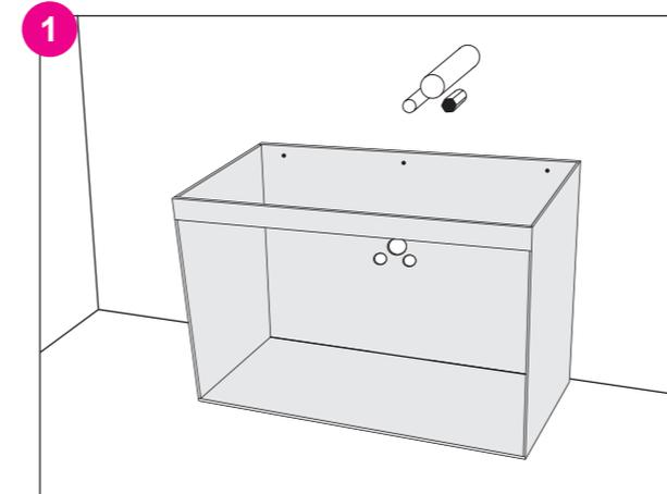
Remove doors & drawers and drill holes for plumbing in the back panel and/or base of the cabinet with an appropriate sized hole saw. Pre-drill screw locations for fastening to wall in step 4
