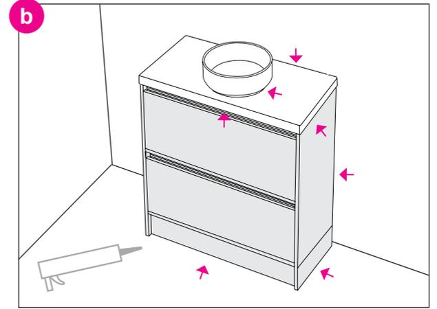
When sealing a vessel or semi inset basin it is important to put a bead of silicone around the edge where the basin meets the top. As well as where the top meets the wall.
