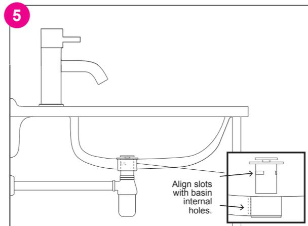
When fitting waste to basin do not overtighten or the basin may be damaged. Use suitable overflow waste and align the slots with the internal holes. Ensure that no excess silicone or putty is obstructing the water flow.
