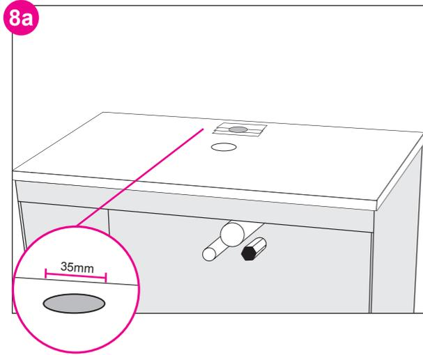
Decide on the location of your taphole and measure out position. Tapholes should be drilled with a sharp Bi-metal hole saw. The drilling is done in three steps. Cover the area you plan to drill with masking tape. Drill a pilot hole through the counter top at your center point. This hole should be just slightly smaller than the size of the pilot bit of your hole saw.
