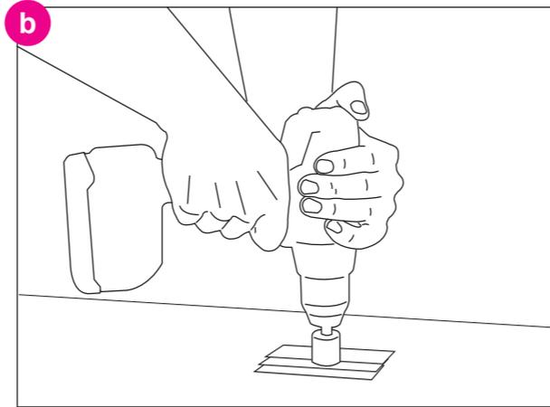
Using this hole as a guide, use a sharp hole saw to cut the hole to 35mm for a standard taphole size.
