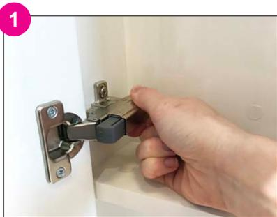
To separate the softclose mechanism from the hinge use two fingers and gently pull from the back to the front.
