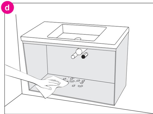
Clean away all building residue from the cabinet. Take care to dry any spillage or leakage of water on or inside the cabinet during installation.
