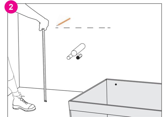
Mark the position of the top of the vanity - factor in the top/ basin thickness to get the correct height. Use a single screw in center of vanity to hold it in place.
