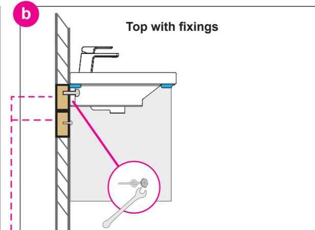
3. If installing a basin with bolt fixings - ensure basin is fixed into nogs with supplied fixings as well as using a silicone sealant to the top of the cabinet.
