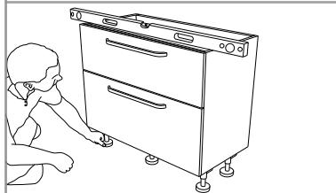
Ensure that the adjustable legs are pre-set at 150mm before installation begins. Measurements are taken from the underside of the cabinet to the floor.
