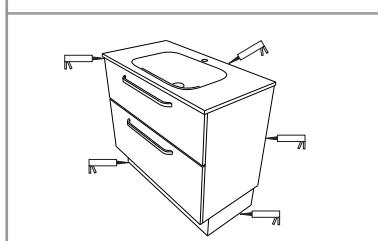
Apply silicone to the top edges of the cabinet and ensure that the unfinished/raw edge of the cabinet sides, front support rail and back are sealed before the top is positioned. Attach the basin to the top of the cabinet with a continuous bead of silicone and then proceed to silicone all the cabinet and shroud edges that are in contact with the wall and floor.
