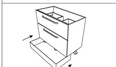
Slide the stainless steel shroud into place. Push until the front of the shroud sits firm against the front legs and the back of the shroud is flush with the back of the cabinet.
