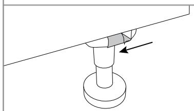
Prepare double sided tape, located on the rear left and right legs, by peeling the protective layer off and exposing the adhesive.
