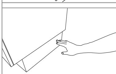
When it is in place, push the back left and right ends of the shroud against the double sided tape located on the rear legs.
