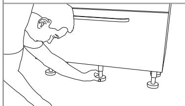
When the cabinet is level unwind the middle leg clockwise until it touches the floor.
